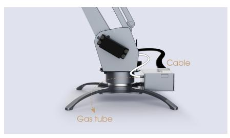
Step 2.2 - Attach the Cable and the Pipe
