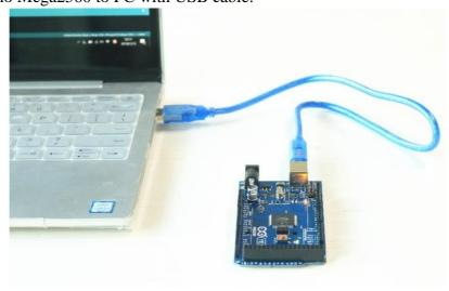
(3) Open the firmware with Arduino IDE, set the parameter as below, click"Upload" to upload firmware to Arduino Mega2560.
