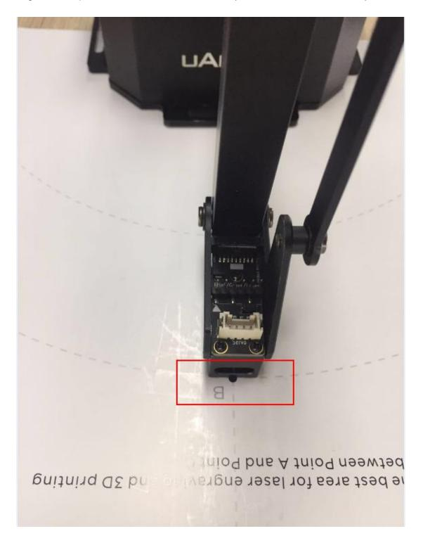
3.8 Type in "M2401 B" in the command box and click send to calibrate. Calibration is done when it returns "ok"
